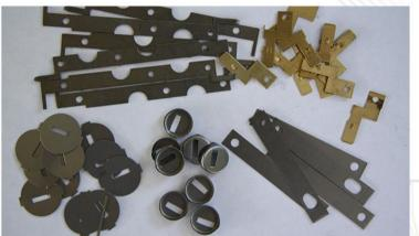
UPRZ carries out cold stamping of sheet (including the roll one) material, thickness of which may vary in the range of 0,3-6 mm, in presses with pressing force of up to 160 tf.
