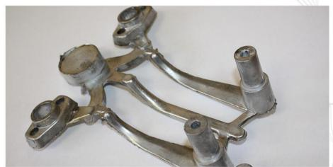
On UPRZ there is a site equipped for casting under pressure of metal alloys based on two types of metals: aluminum and zinc.
