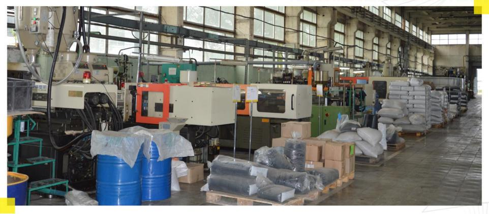
Plastic molding is carried out at the plant using the equipment made by leading foreign manufacturers: «Battenfeld» (Germany), «Arburg» (Germany), «Bole» (China).
